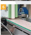
Hot-foil or thermal transfer printers can be easily integrated in order to print variable data.
