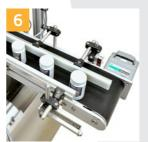
The 152C masters various mounting conditions and production environments. The conveyor belt is available with a width of 100 or 150 mm, at a length of 1,540 mm.
